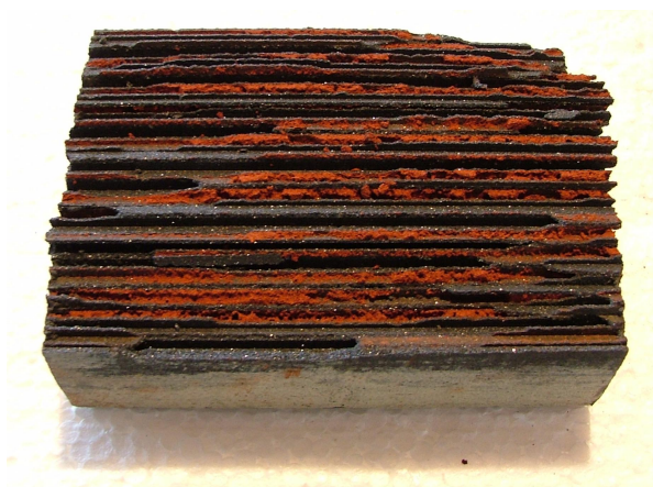
Fig. 4: Clogged ceramic monolith and sinter metal filter package folded apart
